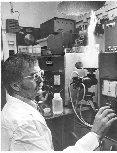
LIAL BREWER (3311) uses the Atomic Absorption Spectrophotometer to check a beryllium sample in the spectrochemistry lab.
